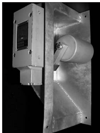
Fig. 6. Typical Limit Switch in mounting housing with bottom at an angle so as to prevent accumulation of material. Unfortunately, the system is not totally fail-safe.
