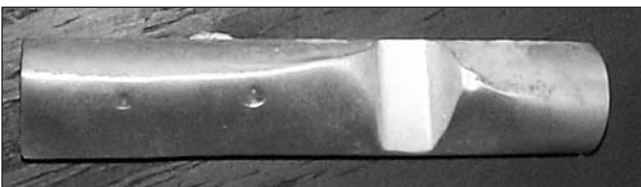
Fig. 5. Bronze plate sensor. Wear due to friction.
