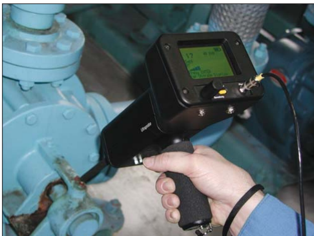
The UE Ultraprobe 10,000, left, can detect bearing failures in the very early stages of failure. In the photo on the right, you can see the predictive technique used in the 1970s for detecting bearing failures, and possibly the fault correction tool.
