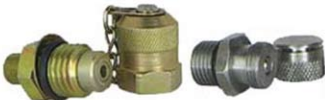
Figure 3. Gauge plug (shown on the left) and flush mount type sample ports for static (gravity flow) and pressurized system sample collection. (Courtesy of Condition Monitoring International)
