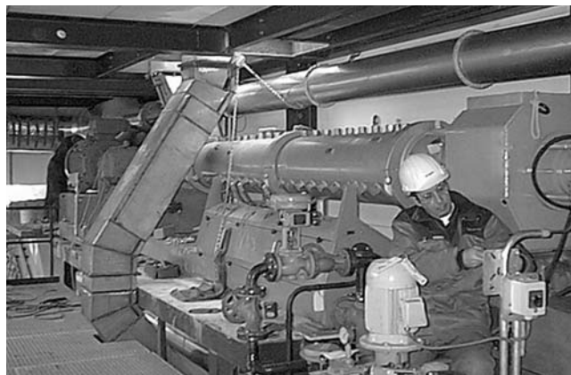
A Tecnal model EXP-350MLE expander with 300 Kw motor sized to process flakes from 1500 mtpd soybeans.
