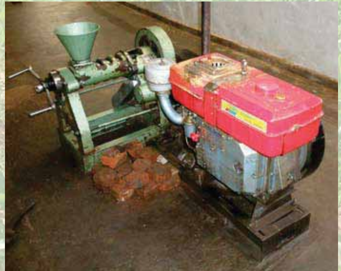
The mechanical screw press used to extract oil from groundnuts (peanuts), sunflower seed, and soybeans at the Mitundo Agro Processors plant in Malawi.
